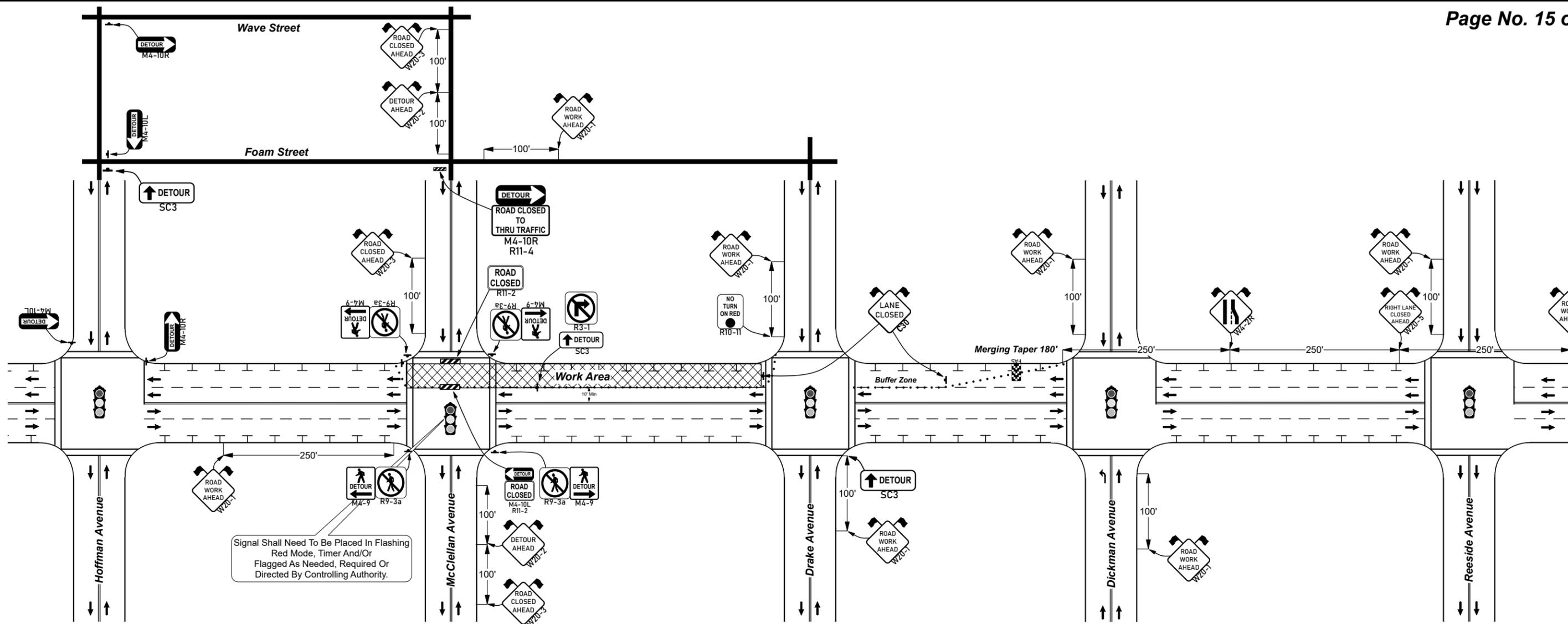
Signal Shall Need To Be Placed In Flashing Red Mode, Timer And/Or Flagged As Needed, Required Or Directed By Controlling Authority.
