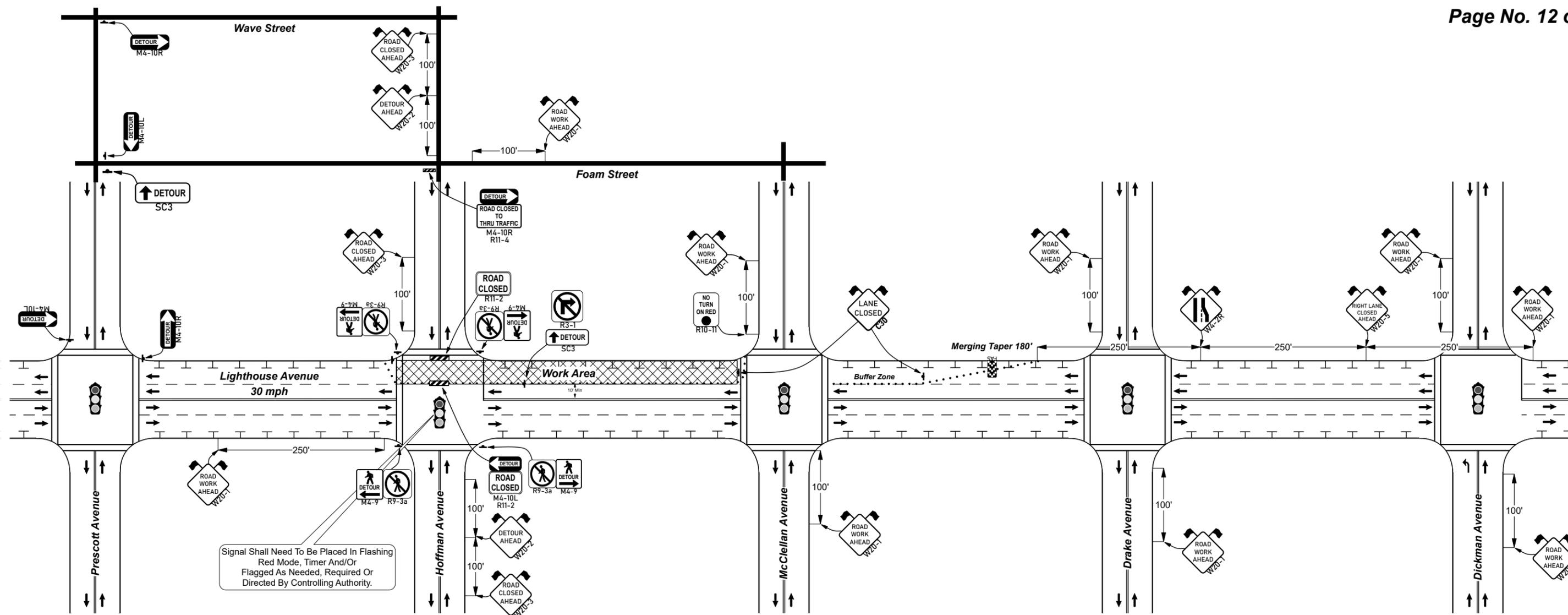
Signal Shall Need To Be Placed In Flashing Red Mode, Timer And/Or Flagged As Needed, Required Or Directed By Controlling Authority.
